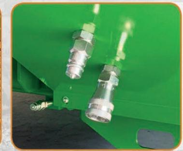
• OPTIONAL USCITE IDRAULICHE PER CONNESSIONE ACCESSORI
