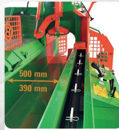
• AMPIA VASCA SPINTORE CON BLOCCAGGIO IDRAULICO SUPERIORE
